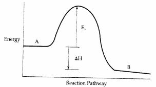
The activation energy in the forward direction,  $E_{af}$ , equals  $E_{u}$ , and the activation energy in the reverse reaction,  $E_{ar}$ , equals  $E_{u}$  –  $\Delta H$ . (The same is true for an endothermic reaction because the sign of  $\Delta H$  is the positive and  $E_{ar}$  <  $E_{af}$ ). For the reaction in question,
