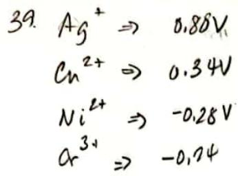
a) largest  $\text{Ag/Cr} \Rightarrow E_{\text{cell}}^\circ = 0.80 - (-0.74) = 1.54\text{V}$
