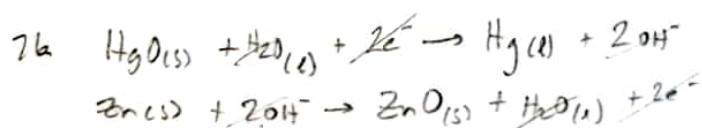
$$E_{\text{red}}^\circ(\text{HgO}) = 0.098\text{V}$$
