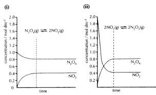
Graph (i) shows the decomposition of  $N_2O_4$ . Graph (ii) shows the reverse reaction starting with  $NO_2$ . Once equilibrium is reached (shown by the dotted line), the composition of the mixture remains constant and is independent of the starting materials.
