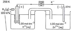
pressure just above 100 kPa so H<sub>2</sub> can escape from electrode
