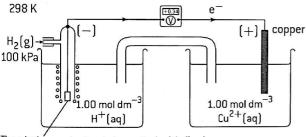
The platinum electrode is coated with finely divided platinum, which serves as a catalyst for the electrode reaction.
