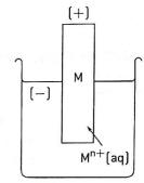
When the half-cell contains a metal above hydrogen in the reactivity series electrons flow from the half-cell to the hydrogen electrode, and the electrode potential is given a negative value. If the halfcell contains a metal below hydrogen in the reactivity series electrons flow from the hydrogen electrode to the half-cell, and the electrode potential has a positive value. The standard electrode potentials are arranged in increasing order to form the
