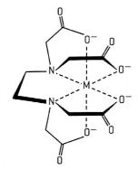
EDTA4- acting as a hexadentate ligand with a transition metal, M to form a complex such as [Cu(EDTA)]2-. Note that the coordination number is still six even though only one ligand surrounds the metal ion.
