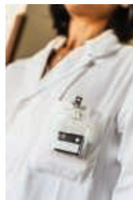
▲ Figure 21.8 Badge dosimeters monitor the extent to which the individual has been exposed to high-energy radiation. The radiation dose is determined from the extent of darkening of the film in the dosimeter.
